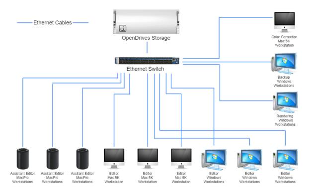
Figure 2. Typical Network Attached Storage (NAS) Architecture
