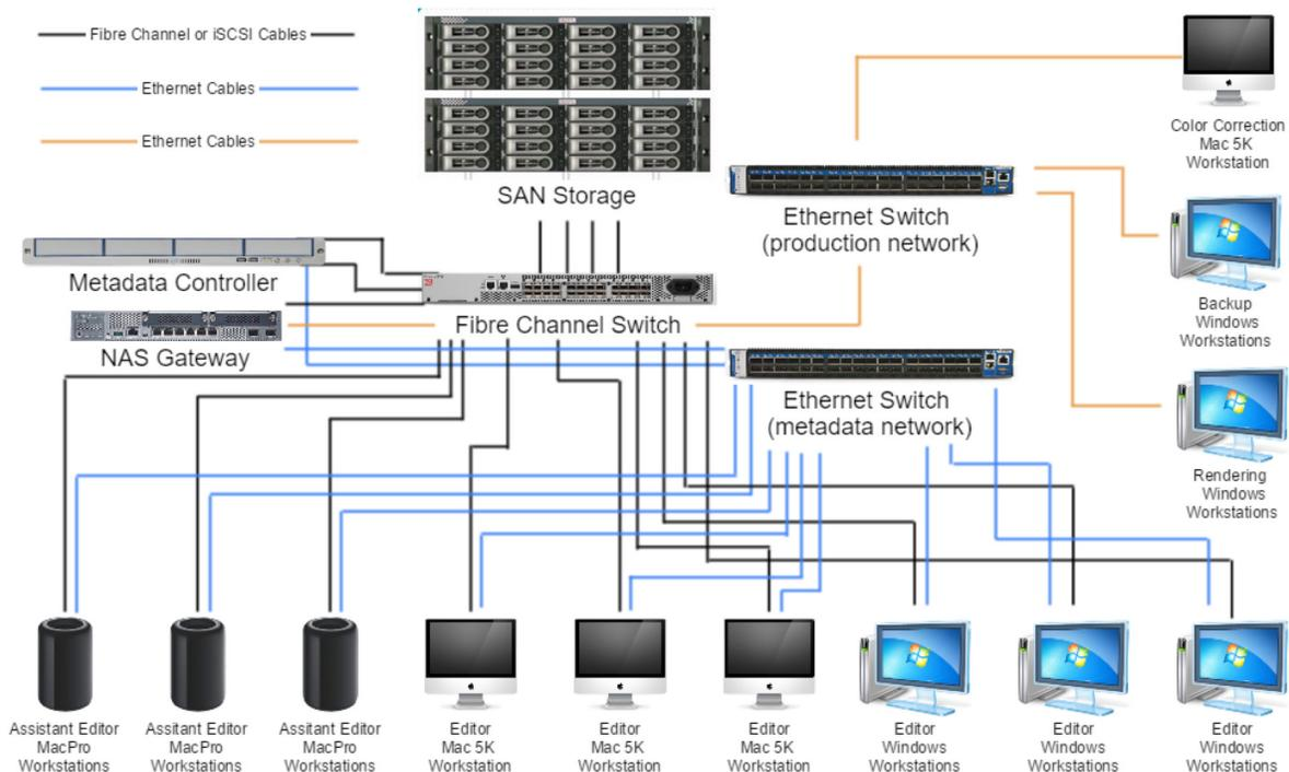
Figure 1. Typical Complex Storage Area Network (SAN) Architecture
