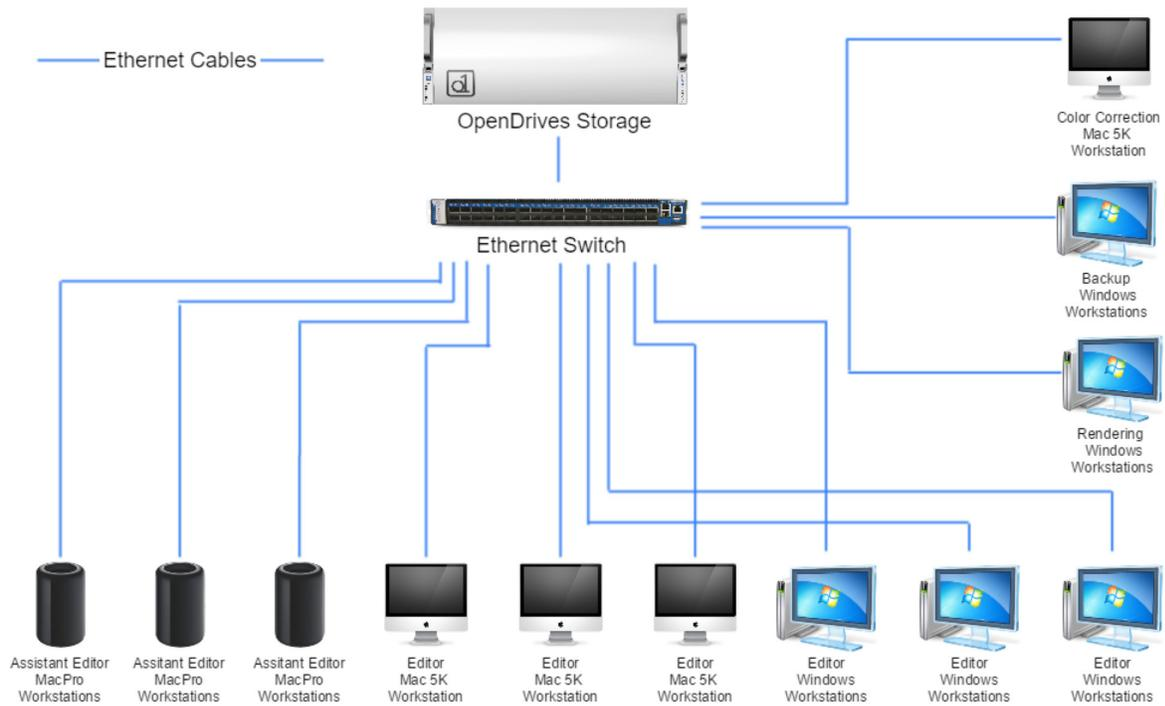
Figure 2. Typical Network Attached Storage (NAS) Architecture
