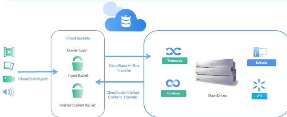
CloudSoda enables direct ingestion of raw assets into cloud storage for protection and leverages cloud tools like transcoding. Users can pull hires or proxies to OpenDrives for editing and push finished content to the cloud, streamlining the workflow and optimizing efficiency.
