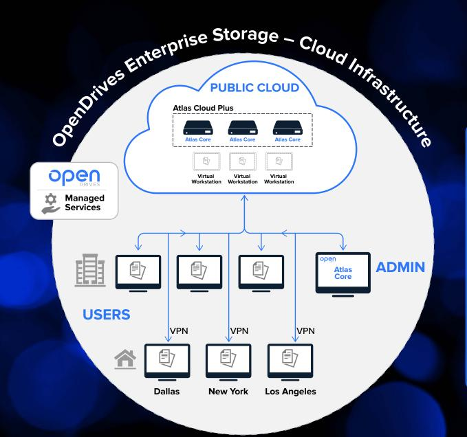
This illustration shows the component parts of OpenDrives' cloud solution, Atlas Cloud Plus, with Atlas Core creating and managing virtualized storage in the public cloud, geographically distributed users accessing the data, and the managed services delivered by OpenDrives who deploys the solution and provides ongoing management and optimization support for customers' data environments.
